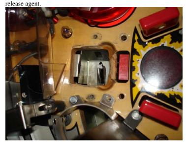
I am lucky that mine did not need the post holes filled as I did on the SOL install. Test the fit the Cliffy protector and prepare to build up the wood where needed. In this case I will need a complete build up behind the drop target and a little on the sides.
