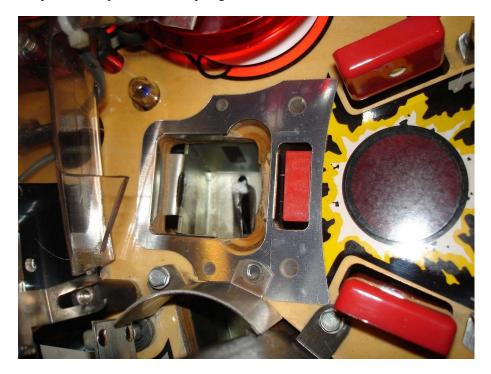
I use a Kraft Mac and Cheese box to make a cardboard mold. It has a nice shiny side that won't grab the filler as easy but a release agent would help. I decided to leave the drop target in place rather than remove. I used the target itself to wedge my cardboard mold against. Your repair may be different.
