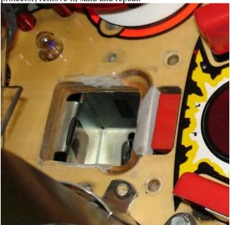
Now put the protectors in place. Make sure you center the moving target protector for best apearance. For the ship protector I put the posts in to line it up, but I did not tap them down tight at first. Screw the left ball guide down, install the three sided ball deflector and when everything is lined up in place tighten and tap posts down flush.
