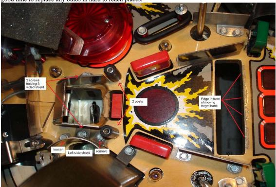
Clean the area pay attention to the two post holes. If these were very tight and squeezing the wood for years it may have created a divot that will need to be filled. Otherwise the tightening of the post may warp the Cliffy protector.
