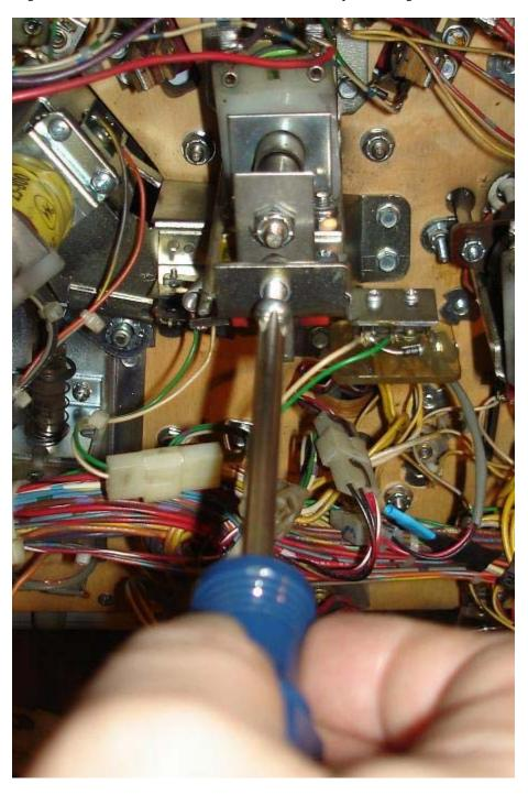
While the playfield is up you can put the nuts and washers back on the posts, tighten but don't over tighten. Make sure the target edge protector is centered and if needed attach with  $\#4 \times 3/8$  screws.
