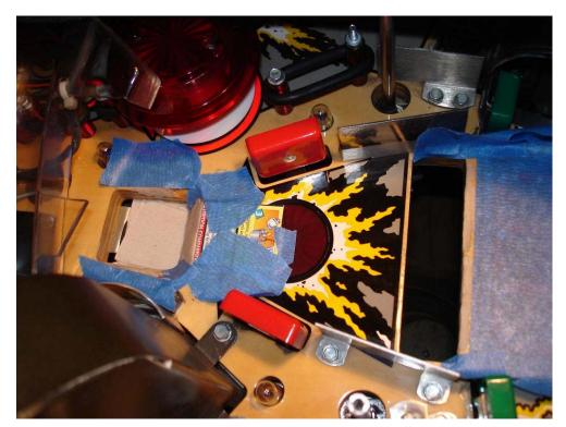
When it is dry, 8 to 24 hours, it can be sanded. I waited 24 to be safe. Cliffy notes he has sanded his repairs within a half hour but the thickness of the repair determines the curing time. I do not feel any of this repair work will be visible so I am not painting. Sand any bumps that will cause the protector to not seat flush. Try the
