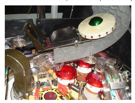
Remove the two Martians and the mothership plastics. If you are like me and have not shopped the machine yet you might be getting your first view of the full damage. Next remove the three sided metal ball guide (deflector) that surrounds the scoop hole (two screws). To the left of the hole you will find another shield. One screw must be removed and the other loosened to allow the protector to slide under. This is also might be a
