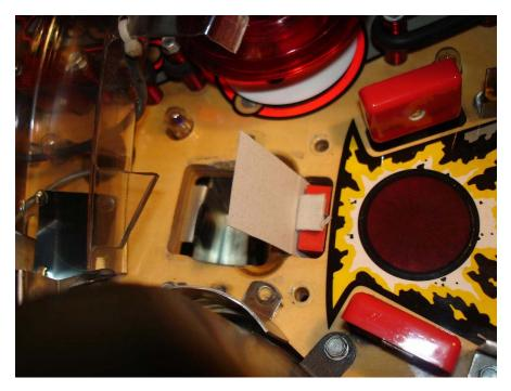
For my repair the cardboard for the front of the ramp was the only mold. I use blue masking tape on the good wood for clean lines and easy sanding without leaving a sticky residue. Use caution, tape can pull up loose paint, stickers and poorly installed insert decals.
