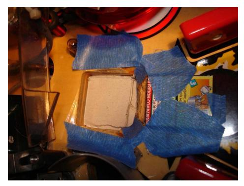
I am using Quick Wood epoxy to fill. A pinball sized dough ball would be more than enough. Push the epoxy against the mold, to the sides of the scoop hole and in front of the moving target bank. I squeeze it in as close as I can to reduce sanding using my fingers, a plastic spoon or putty knife.
