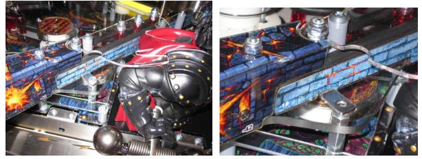
Remove the metal post along the back left side of the upper PF with a ¼ inch nut driver.
