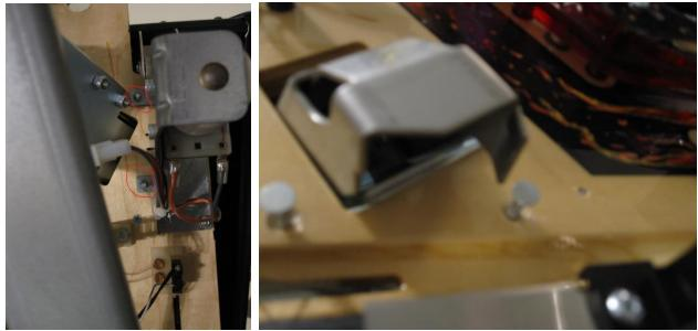
Now you can place the protector and replace the bolts and nuts with the protector in place. DO NOT OVERTIGHTEN! I have had one of these bolts snap in half without a lot of pressure plus you risk warping the protector. Just snug them down flush and you're good.
