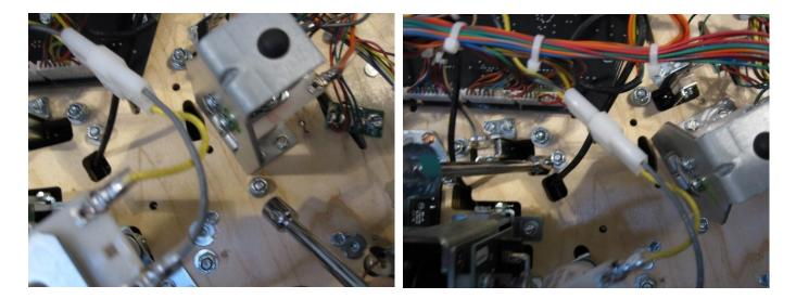
Use included alcohol swab around the VUK. Slip the protector in with the adhesive backing peeled off and then press it in place. Again, clean all the areas of the playfield that you normally can't access and then reassemble the VUK area.
