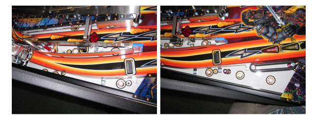
Now remove the 2 metal rails with mostly surface screws and one bolt through the playfield. I suggest thoroughly cleaning this area of the playfield while you are here as you have excellent access. Note that if you use Novus 1, you will then need to use the alcohol wipe provided to then wipe down the small patch of the playfield in front of the kickout hole where the protector adhesive attaches. The adhesive will not adhere to wax in the Novus 1.
