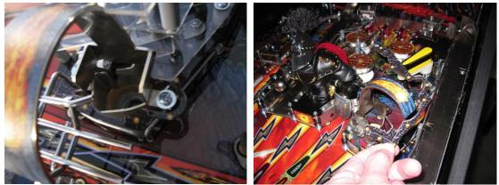
Now remove the curved scoop that takes the ball from the VUK to the wireform ramp that you just removed. There are 2 bolts under the playfield, one screw in front of the scoop and 1 bolt to the right of the knight. Also disconnect the wire connector under the playfield.
