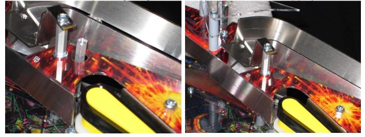
Now you can lift the upper playfield up and out, carefully feeding the cables through the holes in the back panel. Set all the parts you just removed safely out of the way. The flipper stays in place. The white flipper bat shaped plastic beneath the flipper rotates freely and you will need to have this in position beneath the flipper bat itself when you re-assemble the upper PF.
