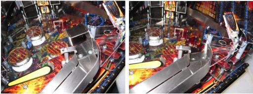
Remove the single screw on the left side of the Knight figure in front of the upper PF.
