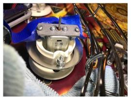
Once the motor is tightened you can put the pirate back on top and use the allen wrench to secure him.
