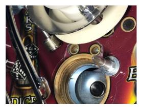
Now use a ¼" deep socket to remove the mini-post. Use the alcohol swab provided in Cliffy's™ kit to wipe around the kickout where the 3M tape will be sticking down. The alcohol is not just a cleaner but also activates the adhesive, along with pressure, so wipe down just when you're ready to install the protector
