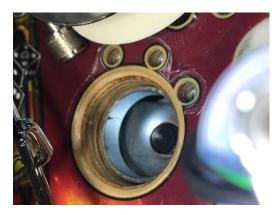
Ready? Peel the protective clear film on top of the protector and then peel the backing from the adhesive side. Align over the kickout and screw holes and then press hard into place all around the front. I like to use a soft cloth to rub the protector down and clean my fingerprints off at the same time.
