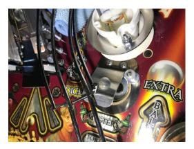
Here comes the fun part © Center the pop assembly back in place and reinstall the two screws in the bottom. Easy. Now I used blue painters tape to hold those stupidly designed white plastic motor spacers to keep them from falling off. Once you get the screws started in the hole you can pull the tape off
