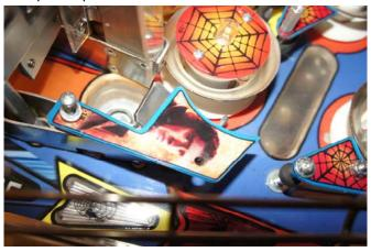
3. Then, lift the playfield to disconnect the Optos (Not shown: they are labeled) and remove the nuts holding the guide lane walls.
