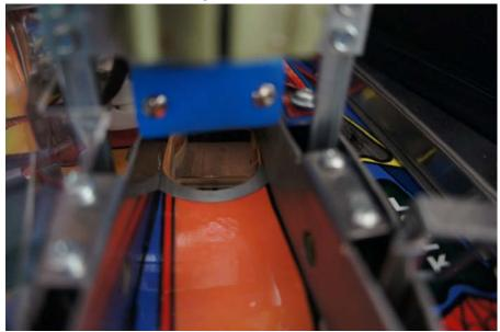
To install the Doc Ock Cliffy protector, you will need to remove the vertical up kicker assembly and the guide walls that contain the Opto sensors.
