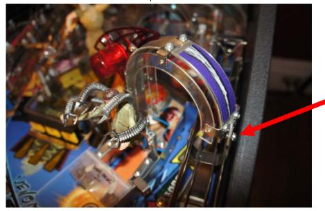
2. Remove the plastics behind the Doc Ock Hole. First remove the clear plastics (not shown), followed by the screened plastic piece.
