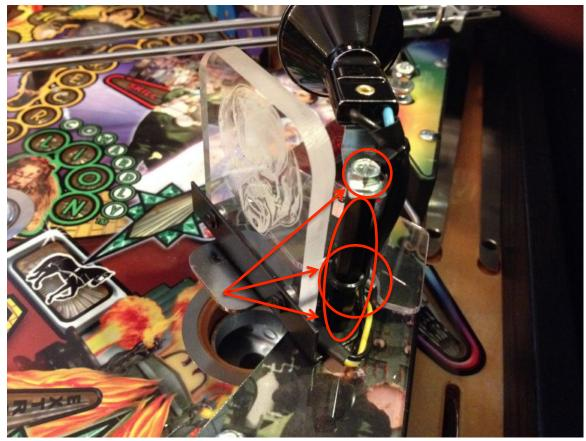
• Next remove the rubber and then two posts. Finally, remove the two screws that hold the scoop down. Use the included alcohol pad to wipe the area the where the Cliffy will be installed. Remove the adhesive, place in position and then press down. Reverse process to re-install everything you removed.
