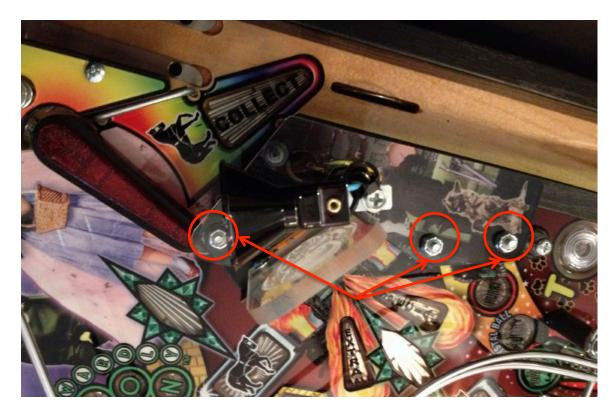
• Cut the wire tie wrapping the spotlight cord and remove the screw and then post as in the pic below. Lay the Wizard to the side and then remove the plastic.
