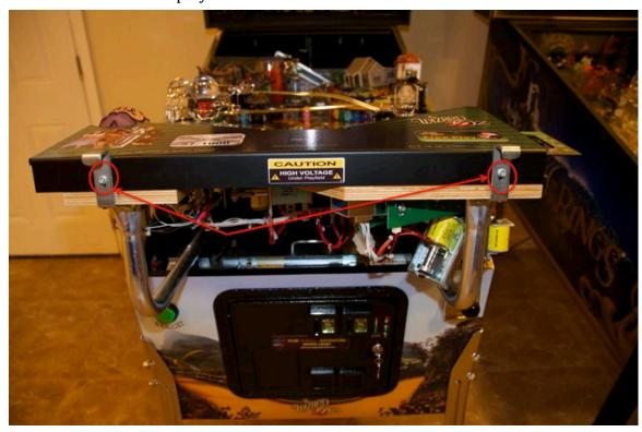
$\bullet \quad$  Remove the two  $\mbox{\em 4}\mbox{\em "}$  screws that attach to the ball trough and ball retainer
