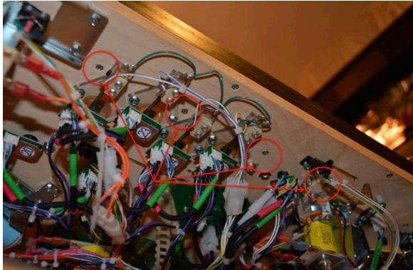
• Lift up slightly on the inner black rail you just loosened and then slide the Cliffy protector under it and then into place. Reinstall screws to ball trough and retainer and then replace screw under PF and tighten the others as well. Congratulations, this one is now done and should like the pic below
