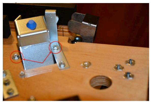
• Loosen, but do not remove four Phillips screws under the playfield that attach to the inner black rail. Remove fully the screw at the farthest left circled in the pic below. This will allow the Cliffy to slide around and in place. If you do not remove this screw, the Cliffy will hit the screw and will not go through.
